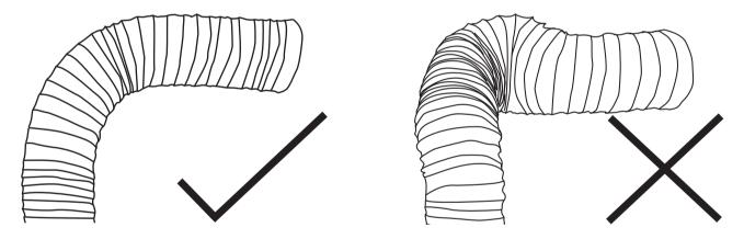
For the Isodrive motors, please do not crush or kink any of the flexi ducting, this will reduce the air flow and may cause noise throughout the system. Ducting needs to be kept taut at all times.
