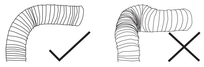
For the Isodrive motor, please do not crush or kink flexi ducting, as it will reduce air flow and may cause noise to occur through the system. Ducting needs to be kept taut at all times. Please refer to the Isodrive motor installation guide for more details on flexi ducting with the silent system.
