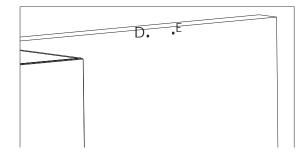
Drill the D, E points with a  $\emptyset$  6mm drill bit to screw the flue installation plate referring to the min. and max. heights of the appliance.
