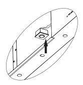
• Before placing the new LED bulb, remove the protective foil on the frame and stick it on its position on the appliance body.
