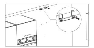
Tighten the flue installation plate to the  $\emptyset$  6 dowels you have tapped to the wall using the 3.9x22 screw supplied with your hood.
