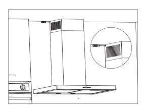
Tighten the inner flue to the flue installation plate secured on the wall from its upper external sides.
