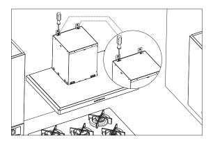
NOTE: If the hood seems skewed, adjust the alignment of the hood by loosening the M5 screws that the suspension plates on the top are installed to.
