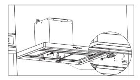
After you have fixed your hood completely, secure the body with a screw from the hole (C) inside the body to prevent it from moving.
