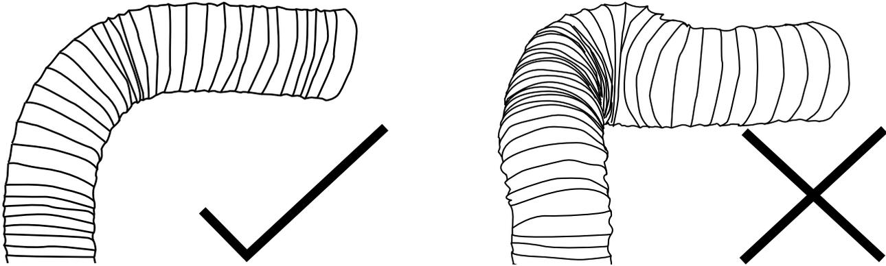
Please do not crush or kink flexi ducting, as it will reduce air flow and may cause noise to occur through the system. Ducting must be kept taut at all times.
