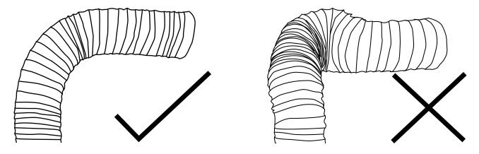
Please do not crush or kink flexi ducting, as it will reduce air flow and may cause noise to occur through the system. Ducting must be kept taut at all times.
