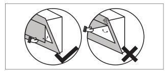
the rangehood (removing the pins from the front guide), ease down slightly and remove. To replace, perform the same operation but in reverse, see figure 2.
