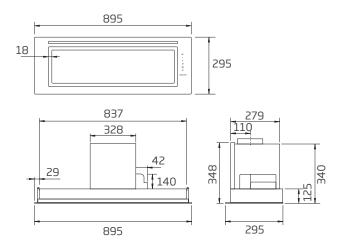
Model:KLS-9GLASS, KLS-9GLASSBLKSFeeding Voltage:220-240V 50HzMax Lamp Power:1 x LED Strip 726mm long<br/>3.36W 12V 4200k
