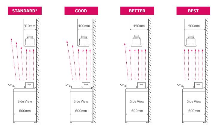
When the overhead cabinetry is constructed and installed deeper than standard, ensure the rangehood is installed as close to the front as possible. This will increase the rangehood extraction results as there is a greater coverage of the cooktop surface area.
