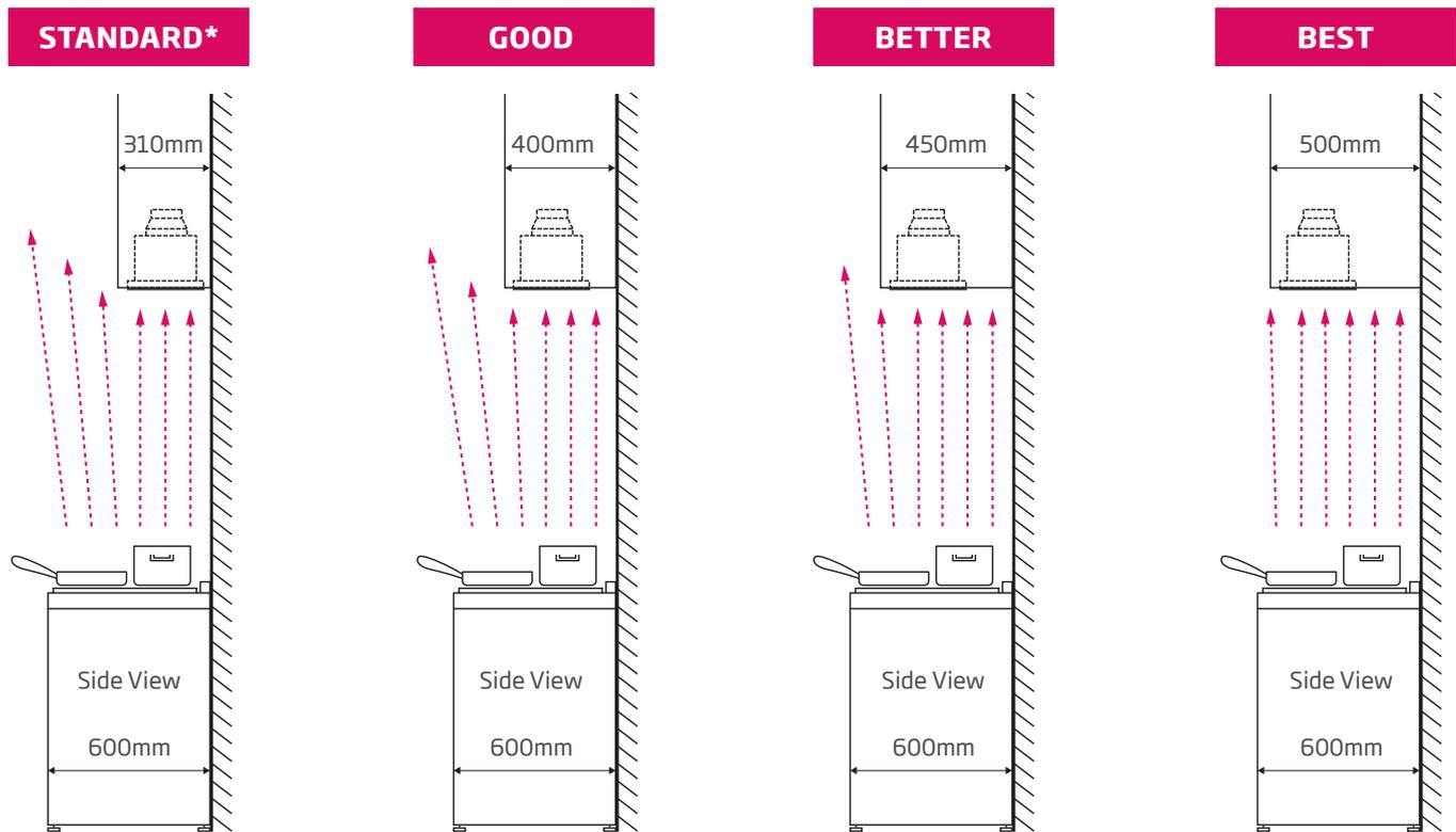
When the overhead cabinetry is constructed and installed deeper than standard, ensure the rangehood is installed as close to the front as possible. This will increase the rangehood extraction results as there is a greater coverage of the cooktop surface area.
