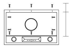
These support screws insert from the bottom of the rangehood.
