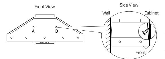
Mounting point A and B need to be tighten with slightly angled screws to pull the rangehood up tight to the cabinet.
