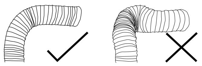
Please do not crush or kink flexi ducting, as it will reduce air flow and may cause noise to occur through the system. Ducting must be kept taut at all times.
